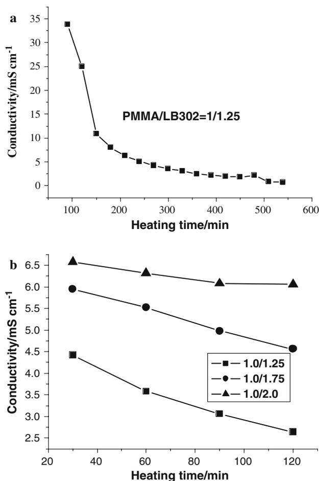
**Fig. 1** Ionic conductivity changes with heating time from in-situ 70 °C measurement and the polymer to liquid electrolyte ratio PMMA/LB302 = 1/1.25 (a) and from intermittent measurements at 17 °C after every half-hour of 70 °C polymerization (b). The PMMA/LB302 ratio is indicated in the graph. Cell system: Stainless steel (SS)/GPE/SS
