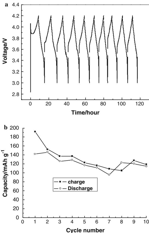
**Fig. 4** Cycling performance of cell LiNi<sub>0.8</sub>Co<sub>0.2</sub>O<sub>2</sub>/GPE/Li at 0.2 mA cm<sup>-2</sup> current density. Cycling curves (a) and capacity-cycle number relationship (b). Here GPE was prepared with PMMA/LB302 = 1/4 and 70 °C polymerization for 2 h
