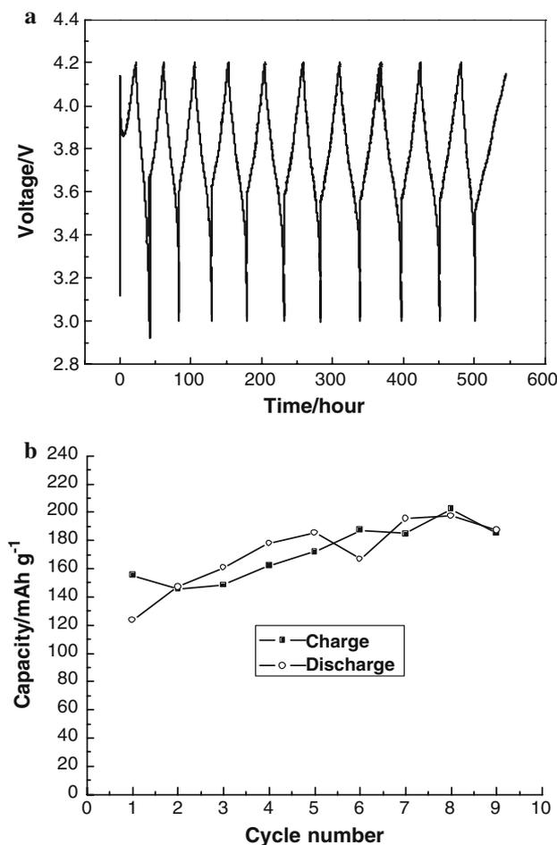
**Fig. 5** Cycling performance of cell LiNi<sub>0.8</sub>Co<sub>0.2</sub>O<sub>2</sub>/GPE/Li at 0.06 mA cm<sup>-2</sup> current density. Cycling curves (a) and capacity-cycle number relationship (b). Here GPE was prepared with PMMA/LB302 = 1/4 and 70 °C polymerization for 3.5 h
