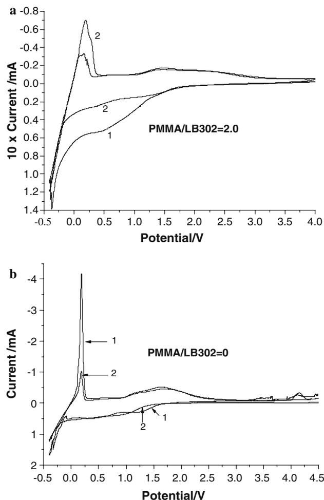
**Fig. 3** Cyclic voltammograms of cells: SS/GPE/Li (a) and SS/LB302/Li (b) Scan rate: 1 mV  $\text{s}^{-1}$
