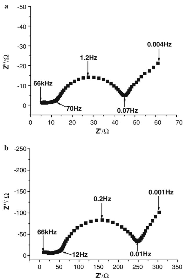
**Fig. 7** AC impedance spectra of a cell  $\text{LiNi}_{0.8}\text{Co}_{0.2}\text{O}_2/\text{LB302}/\text{graphite}$  (a) and  $\text{LiNi}_{0.8}\text{Co}_{0.2}\text{O}_2/\text{GPE}/\text{graphite}$  (b) after three formation cycles. The frequency range was 0.001–100 kHz, electrode area:  $1.54 \text{ cm}^2$  (OCV = 4.0 V)
