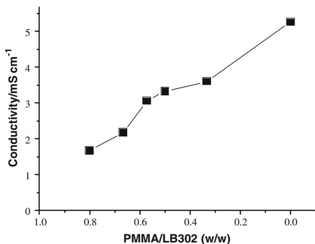
**Fig. 2** Relationship between ionic conductivity of gel-polymer electrolyte and PMMA/LB302 weight ratio. All samples were heated at 70 °C for 2 h and then cooled to room temperature (17 °C)
